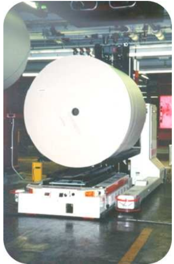
Paper Reel is placed by an AGV onto an Automated Press Loader (APL), which will accurately position the reel into the arms of the reelstand to allow the chuck.
