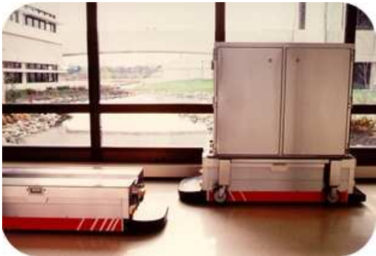
ATLAS vehicle transporting a cart
