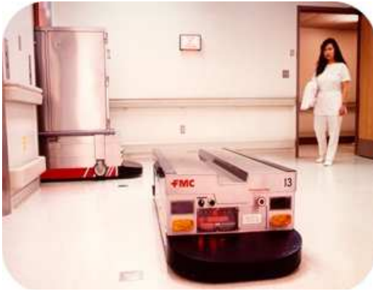
Atlas vehicles delivering carts to patient floors. GMH is a 2 million square feet facility with 1000 beds on the Hospital campus.
