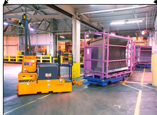
SGV Tugger pulling trailers of stamped F-150 hoods.
