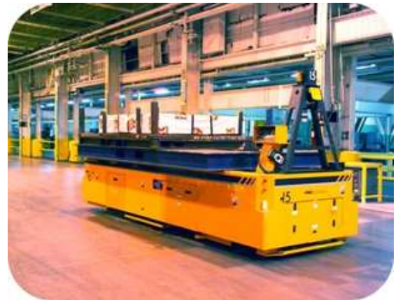
SGV Unit Load Carrying Steel Blanks
